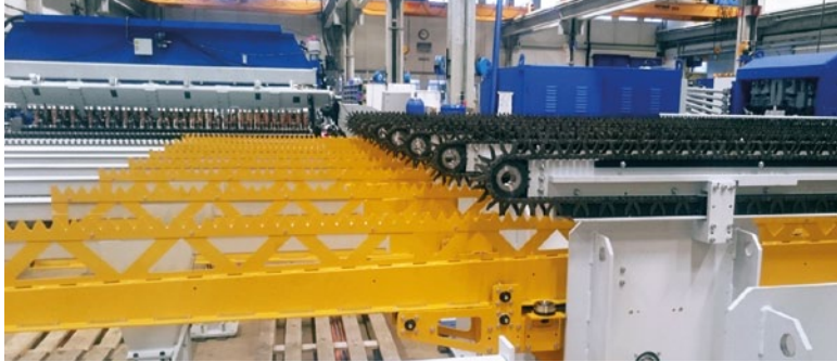
Chain transfer for the line wires
