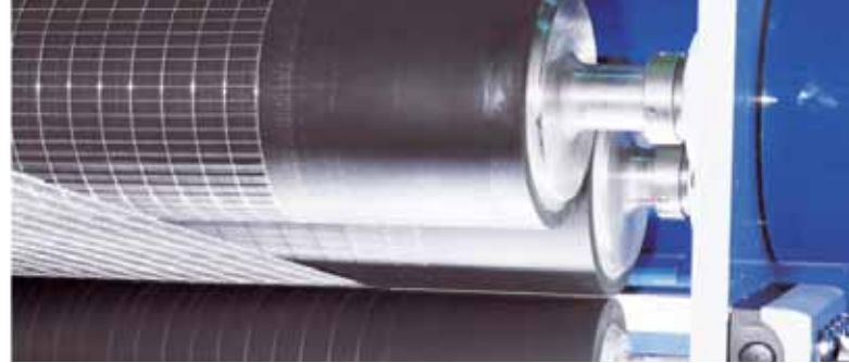
Mesh advance with rubberised 3-roller system
