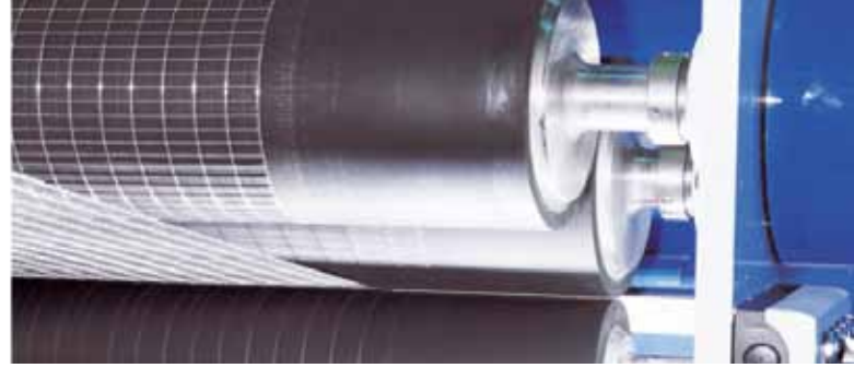
Mesh advance with rubberised 3-roller system
