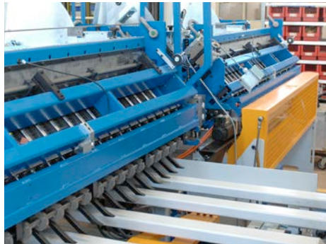
Cross wire feeding device for the upper and lower wire
