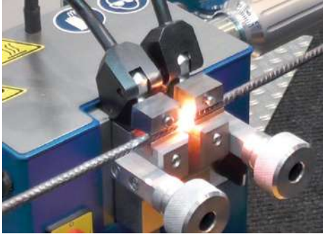
Wire butt welding with consistent high quality
