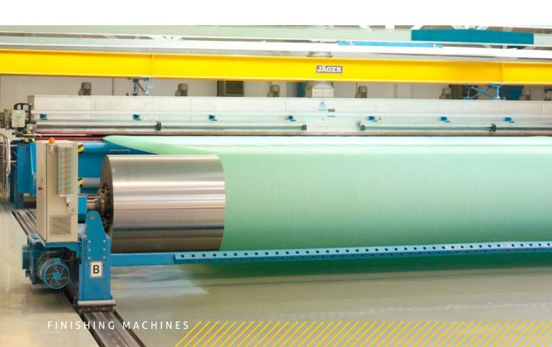
Specially engineered hot-air heat-setting systems with a tenter system with a working width of up to 15 m meet every demand placed on reliable, modern finishing equipment.
