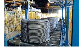
The automatic AVS spooler is supplied with two special automatic collapsible spools and can produce strapped compact coils with weights between 2 and 8 tons and wire diameters between 4 and 25 mm. The special overhead crane manipulator and roll/chain conveyer can be configured according to the customer's plant layout.
