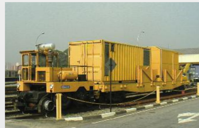
Complete Supra multi flex system with AMS60, mounted onto a rail wagon. Rail welding in the depot.
