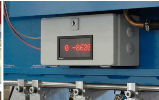
Display for the line wire feed position
