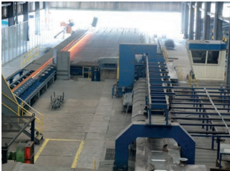
The continuously cast billets are directly fed into the Rolling Mill where they are either rolled to wire and coiled or to straight bars on the cooling bed.
